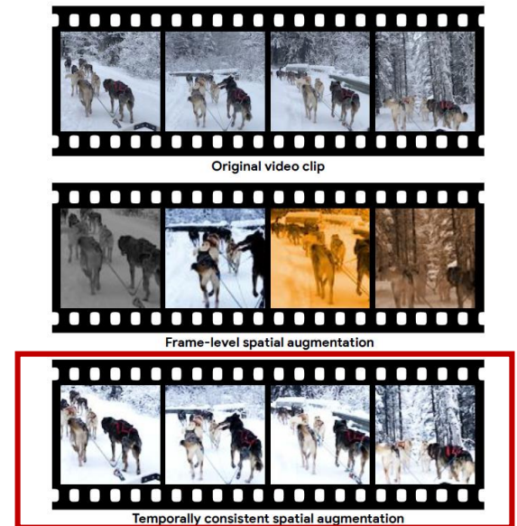
Figure 3. Illustration of temporally consistent spatial augmentation. The middle row indicates frame-level spatial augmentations without temporal consistency which would be detrimental to the video representation learning.
